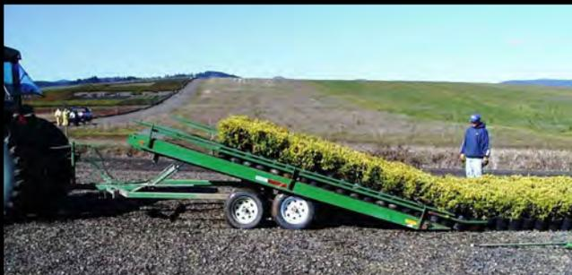
The Drop Trailer allows a full load of containerized plants to fill the bed of the trailer and then be transported to another location. By simply dropping the back end of the trailer, the containers full of plants easily off-load on to the ground in just seconds.
