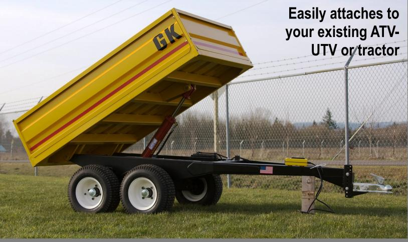
The new GK Dump Trailer has been designed for rugged and heavy duty hauling of field, garden and farm debris. The hydraulic trailer comes equipped with walking beam suspension, on board battery, removable walls and high ground clearance with 18.5" tires. The trailer is powder coated for extra field durability.
